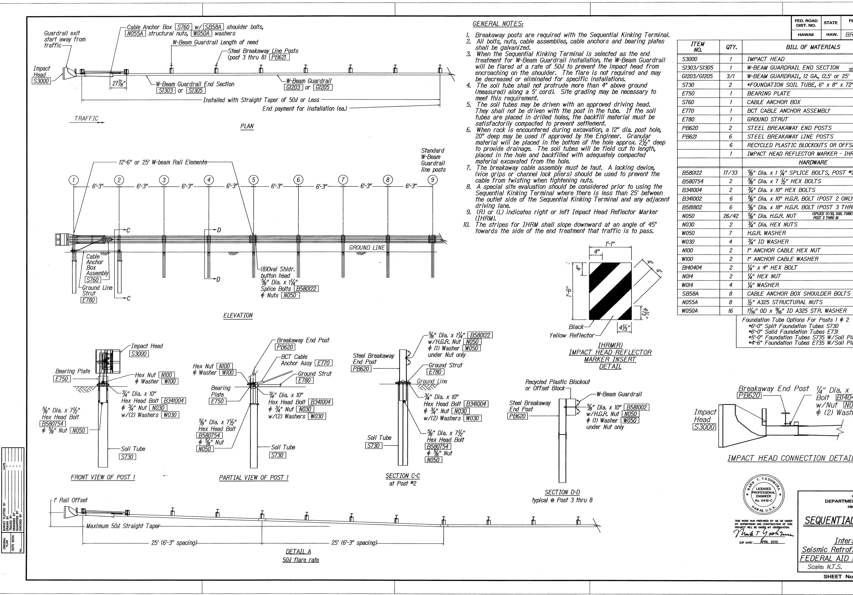
BR-H3-1(79) 2010 BILL OF MATERIALS W-BEAM GUARDRAIL END SECTION W-BEAM GUARDRAIL, 12 GA., 12.5' or 25' \*FOUNDATION SOIL TUBE, 6" x 8" x 72"
