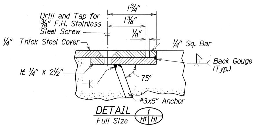
NOTE: All Steel Parts shall be galvanized in accordance with the requirements of ASTM A123.
