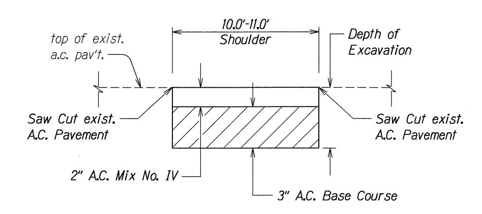
A.C. PAVEMENT RECONSTRUCTION DETAIL Not To Scale
