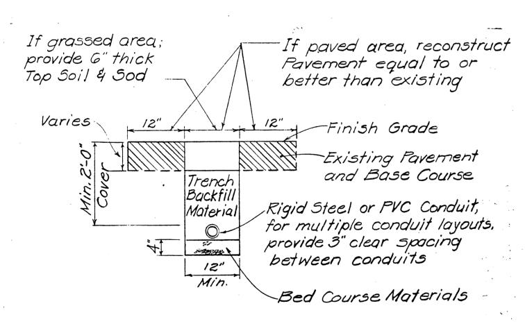
TYPICAL TRENCH SECTION FOR CONDUIT
