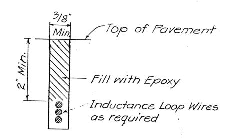
INDUCTANCE LOOP SAW-CUT SECTION A-A (TYPICAL)
