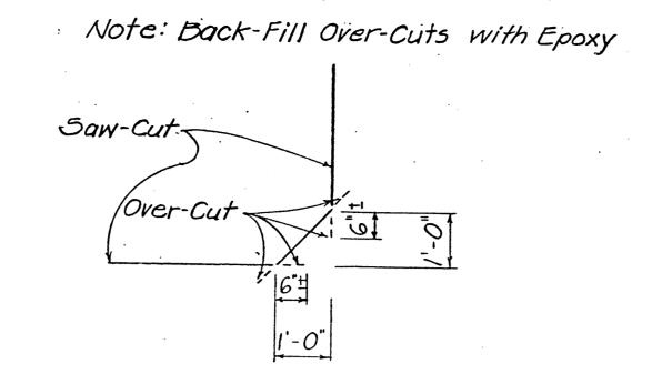
DETAIL B' SAW-CUT AT CORNERS
