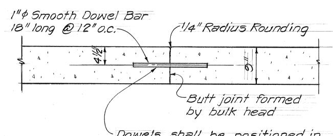
Dowels shall be positioned in place parallel to the pavement surface prior to paving and the ends of the dowels shall not deviate more than 0.02' from the parallel.
