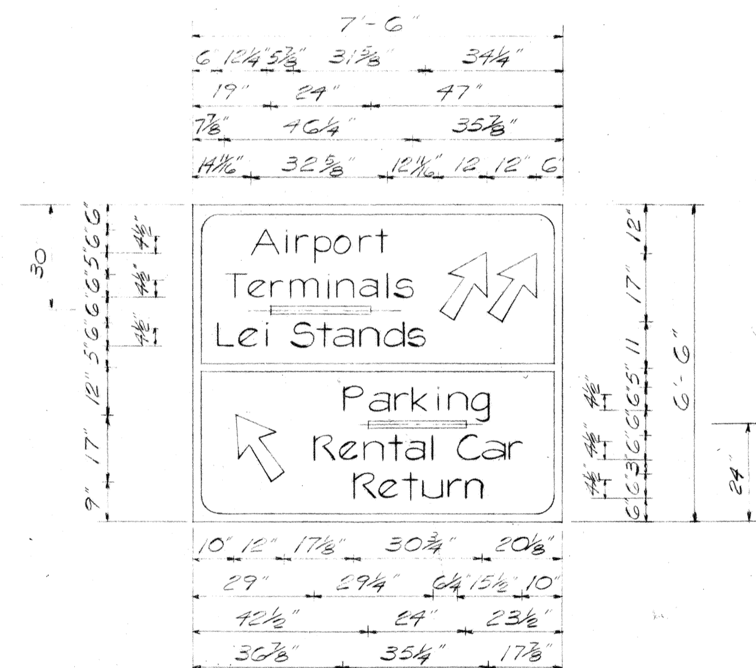
D-5 (Temporary Sign) Scale 1/2" = 1'-0"
