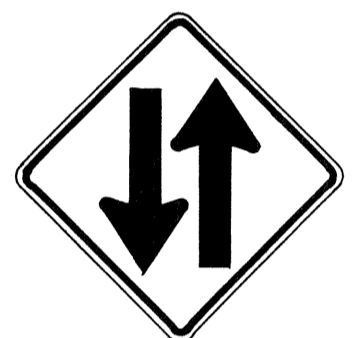
TWO WAY TRAFFIC W6-3 30"x30" 24"x18" W6-3-A 36"x36" 24"x18" W6-3-B 48"x48" 24"x18"
