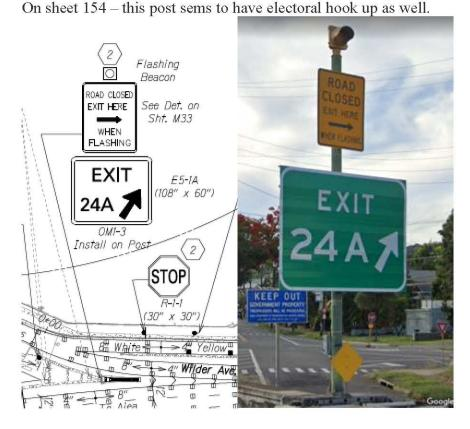
All existing I-Pipe posts and Flashing Beacons shall remain in place. Only the corresponding destination or guide signs will be replaced. Refer to updated Pavement Marking & Signing Plans.
