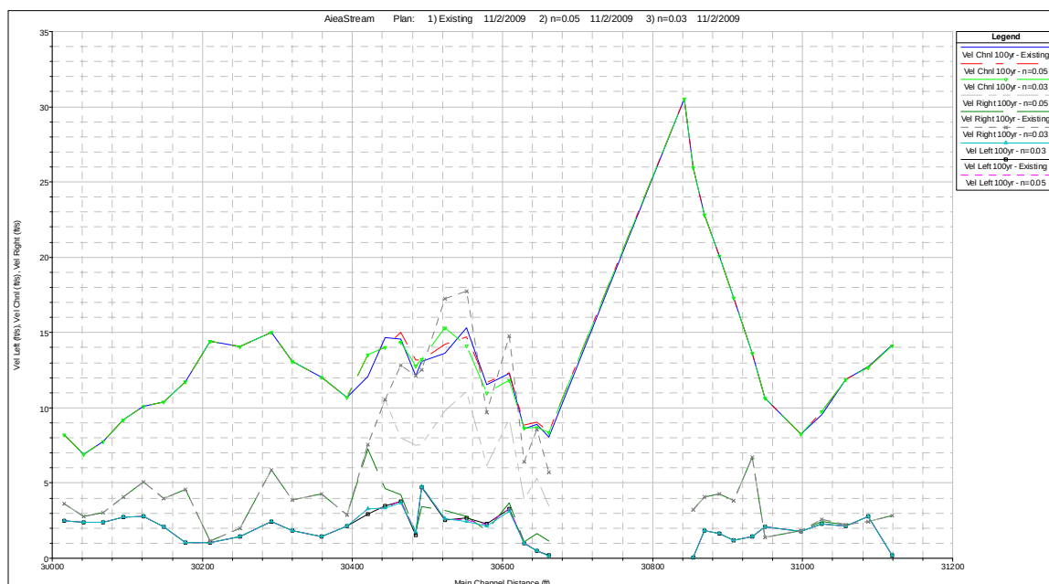
Figure 15. Velocity Profile Comparisons for 100-Year Flood.
