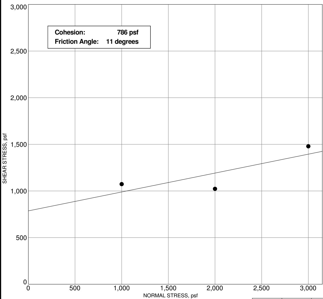
DIRECT SHEAR 8049-00 GPJ GEO LABS GDT 5/3/21
