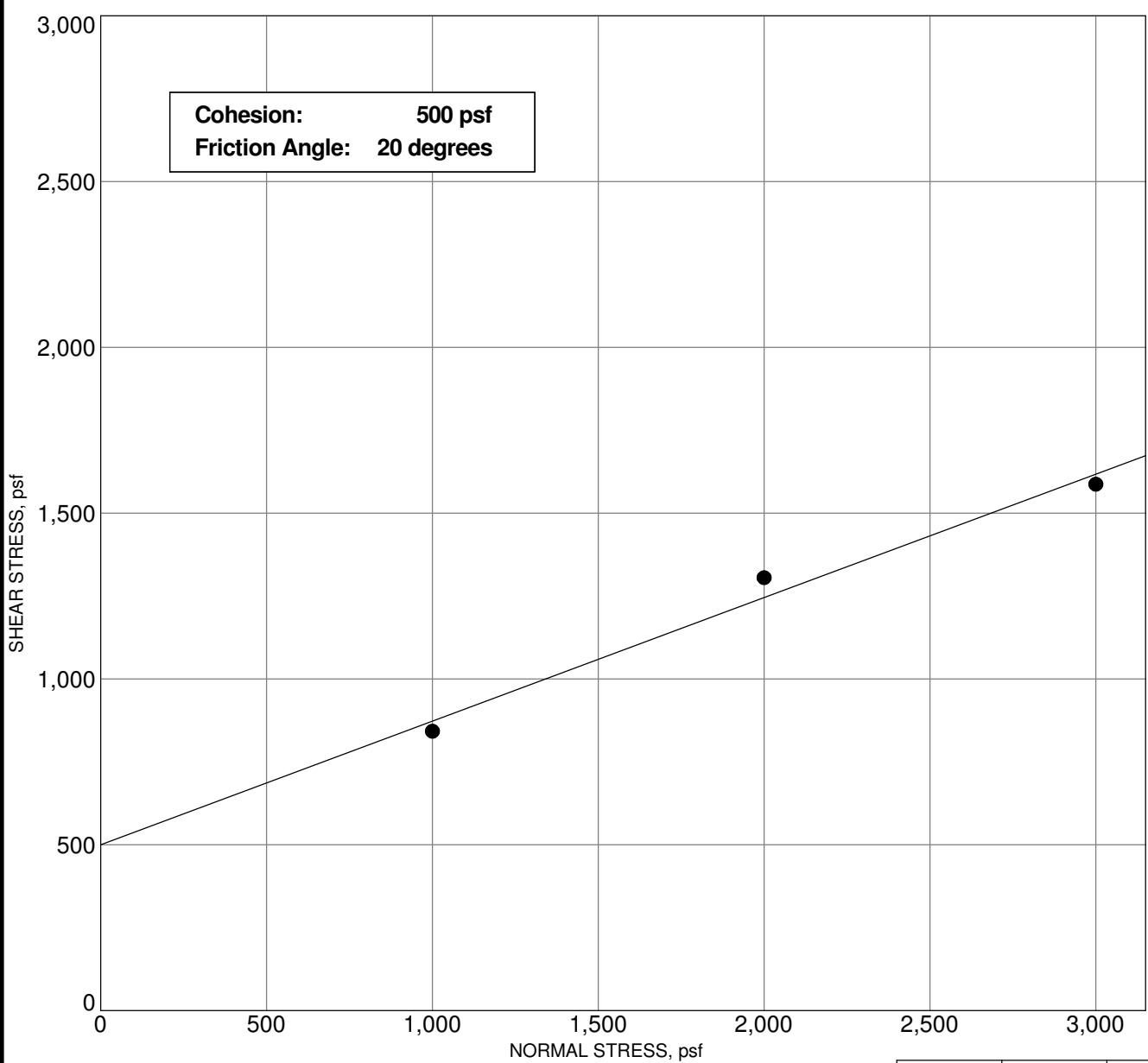
DIRECT SHEAR 8049-00 GPJ GEOLABS GDT 5/3/21
