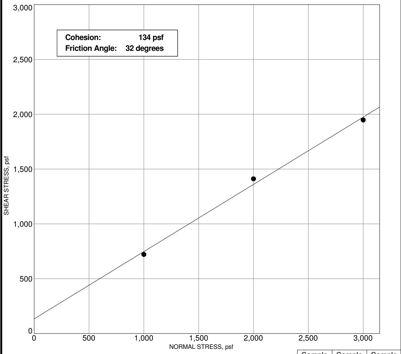
DIRECT SHEAR 8049-00 GPJ GEOLABS GDT 5/3/21
