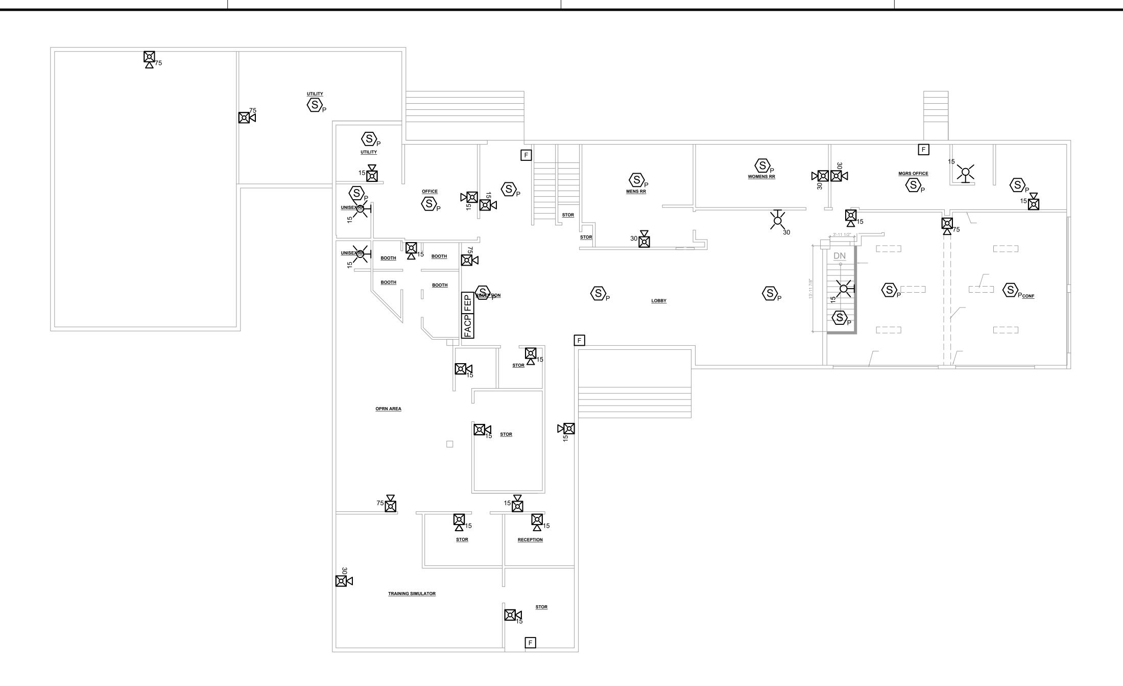
2 ATCT GROUND FLOOR - FIRE ALARM PLAN
