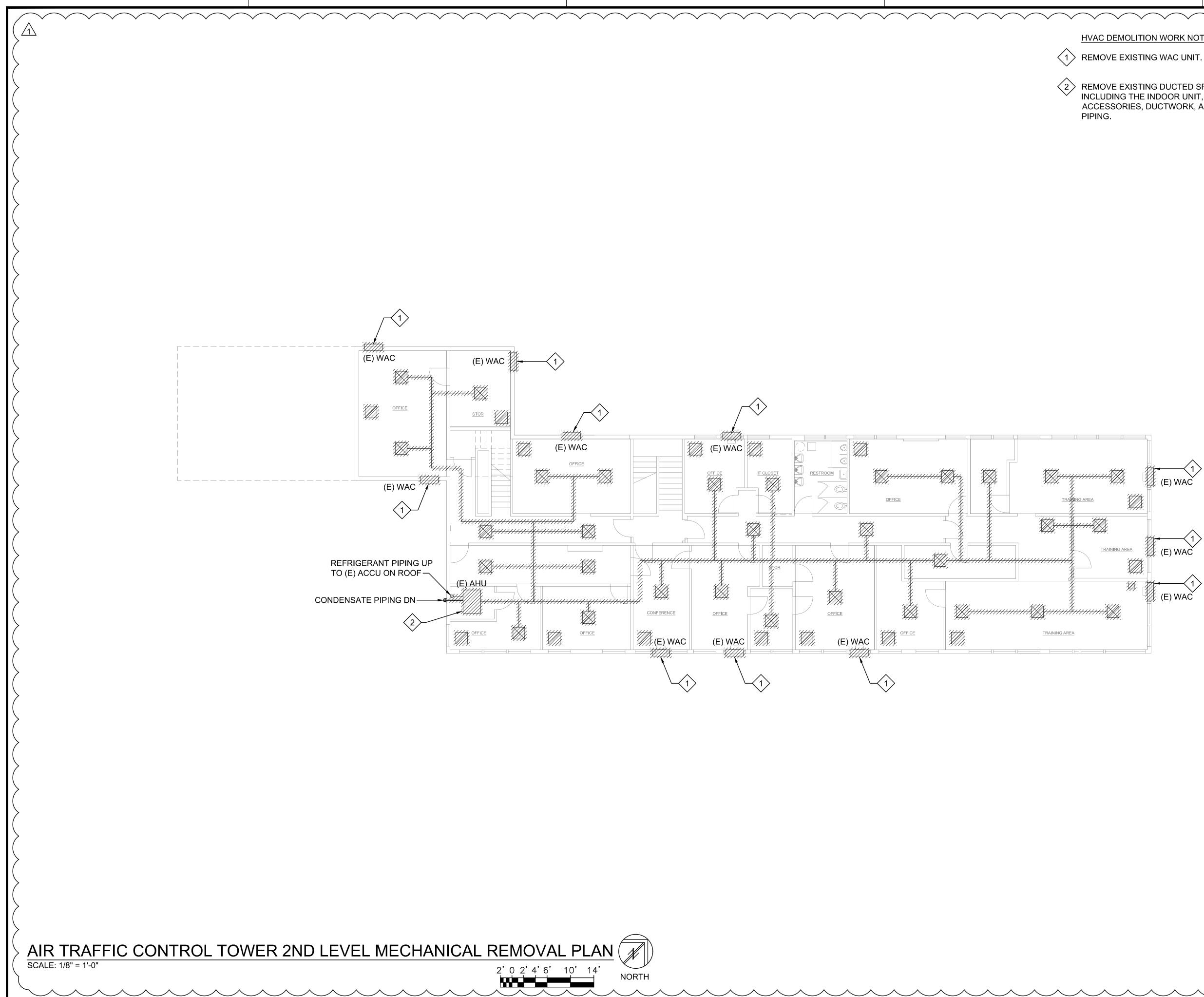
HVAC DEMOLITION WORK NOTES  $\langle 2 \rangle$  REMOVE EXISTING DUCTED SPLIT SYSTEM UNIT INCLUDING THE INDOOR UNIT, OUTDOOR UNIT, ACCESSORIES, DUCTWORK, AIR DEVICES, AND
