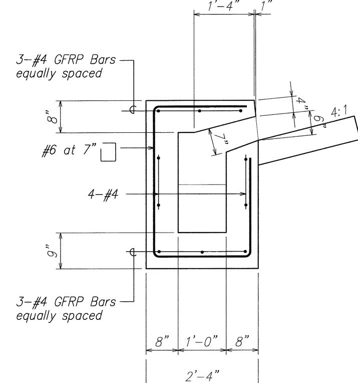
SECTION — CATCH BASIN CURB AND GUTTER
