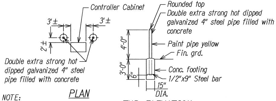
TYP. ELEVATION Cost of conc. filled galvanized PIPE GUARD DETAIL NOT TO SCALE
