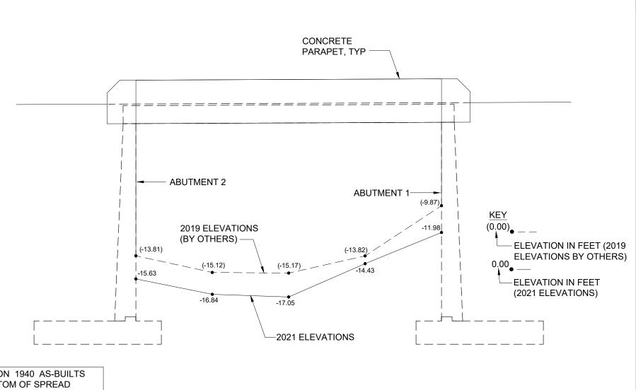
BASED ON 1940 AS-BUILTS BOTTOM OF SPREAD FOOTING ELEVATION:
