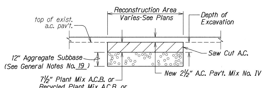
Recycled Plant Mix A.C.B. or Plant Mix Glassphalt Conc. Base Course
