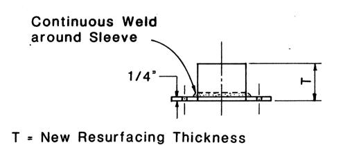
PIPE SLEEVE & PLATE ELEVATION
