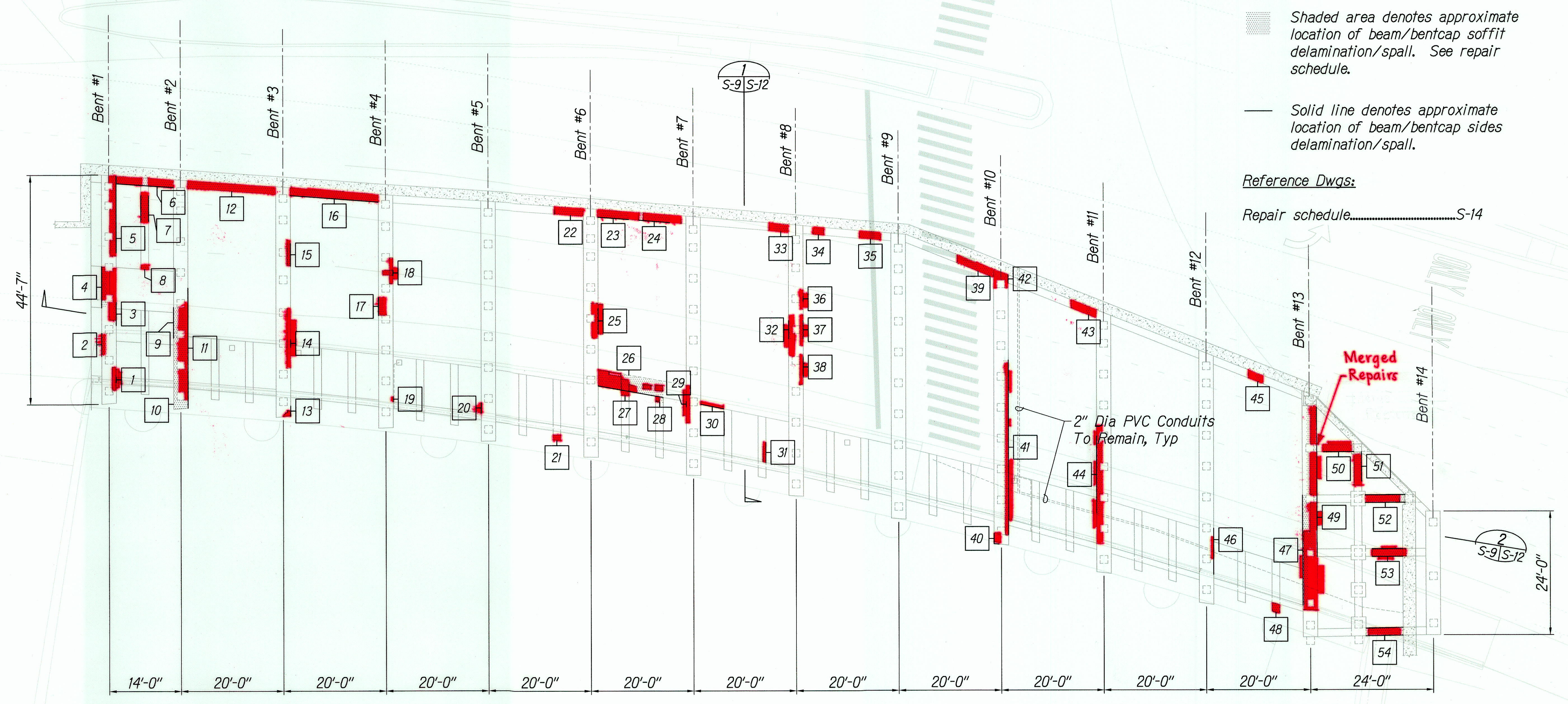
A SLIP COVER #3 BEAM/BENTCAP PLAN S-9/S-9 SCALE: 3/32" = 1'-0"
