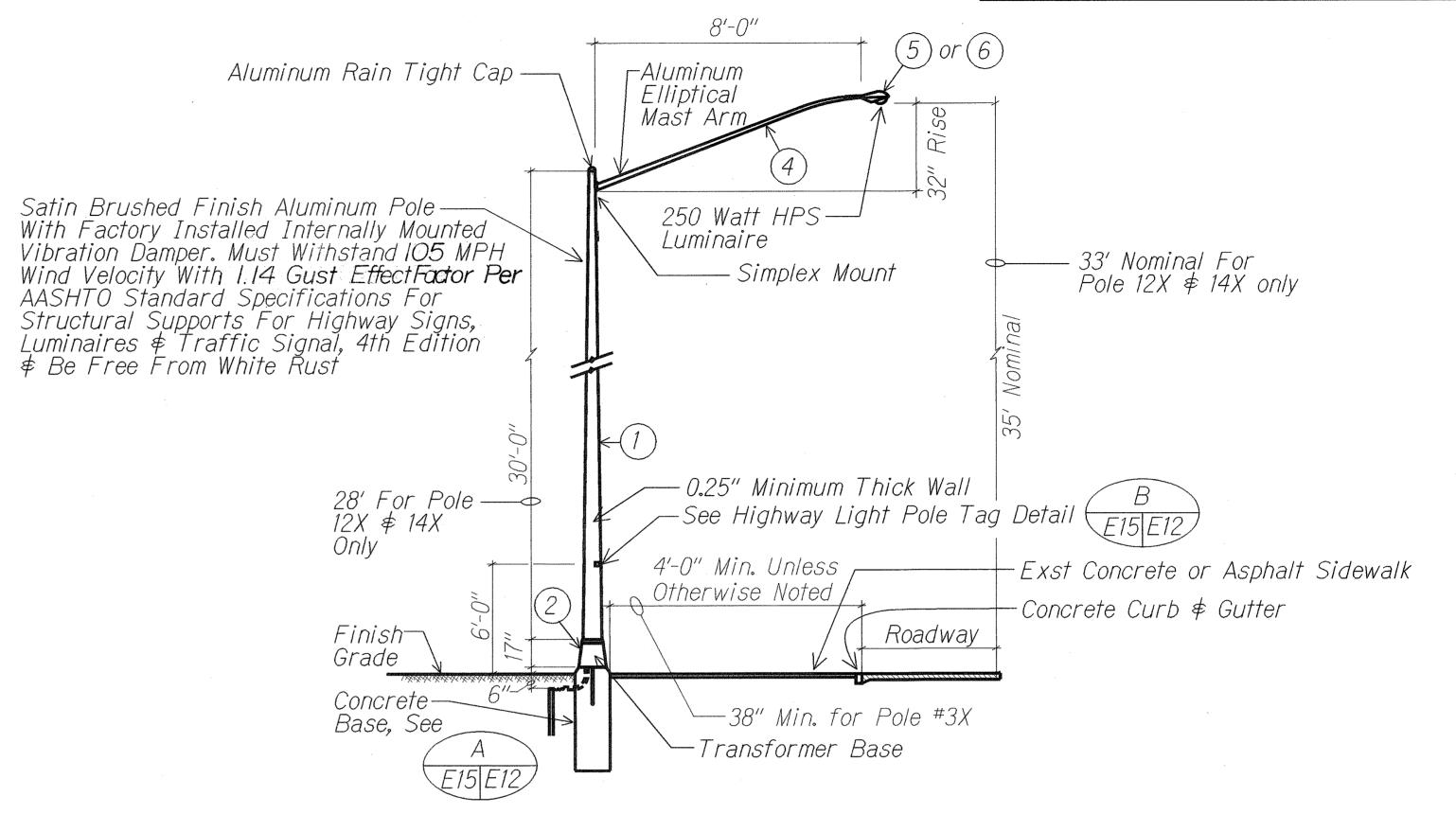
01002-E2 MATERIAL LIST DESCRIPTION ITEM MANUFACTURER Light Pole, 30', Alum Transformer Base (Alum) (Breakaway Type) Mast Arm, 8', Alum, Double Simplex Mount Mast Arm, 8', Alum, Single Simplex Mount Luminaire, 250W HPS Luminaire, 150W HPS
