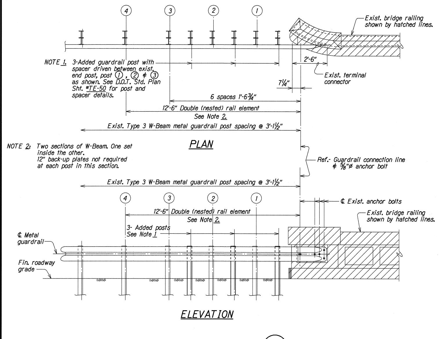
TYPICAL DETAIL (A) LAIEMALOO AND LAIELOA STREAM BRIDGES Scale: 1/2" = 1'-0"
