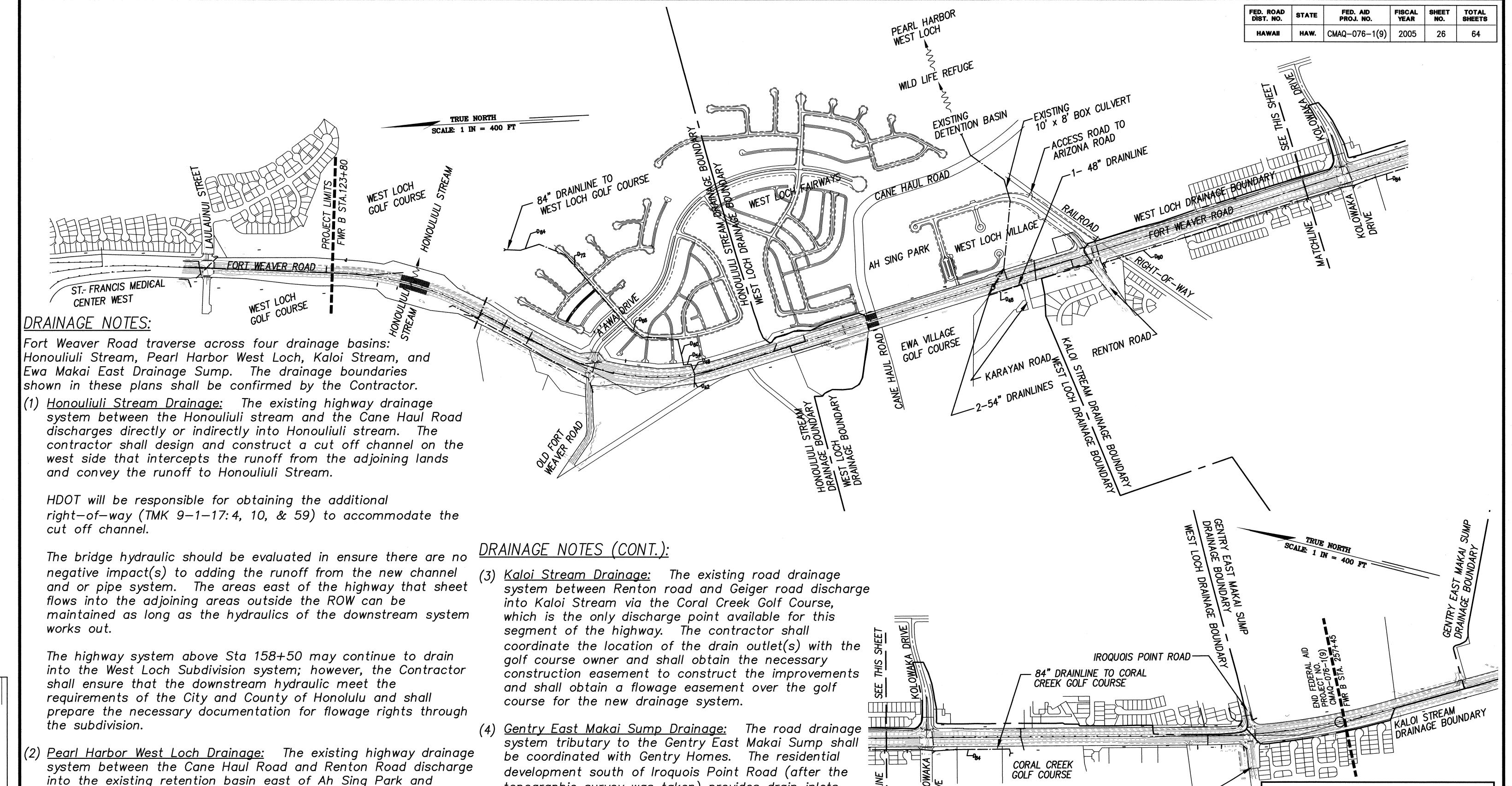
topographic survey was taken) provides drain inlets
