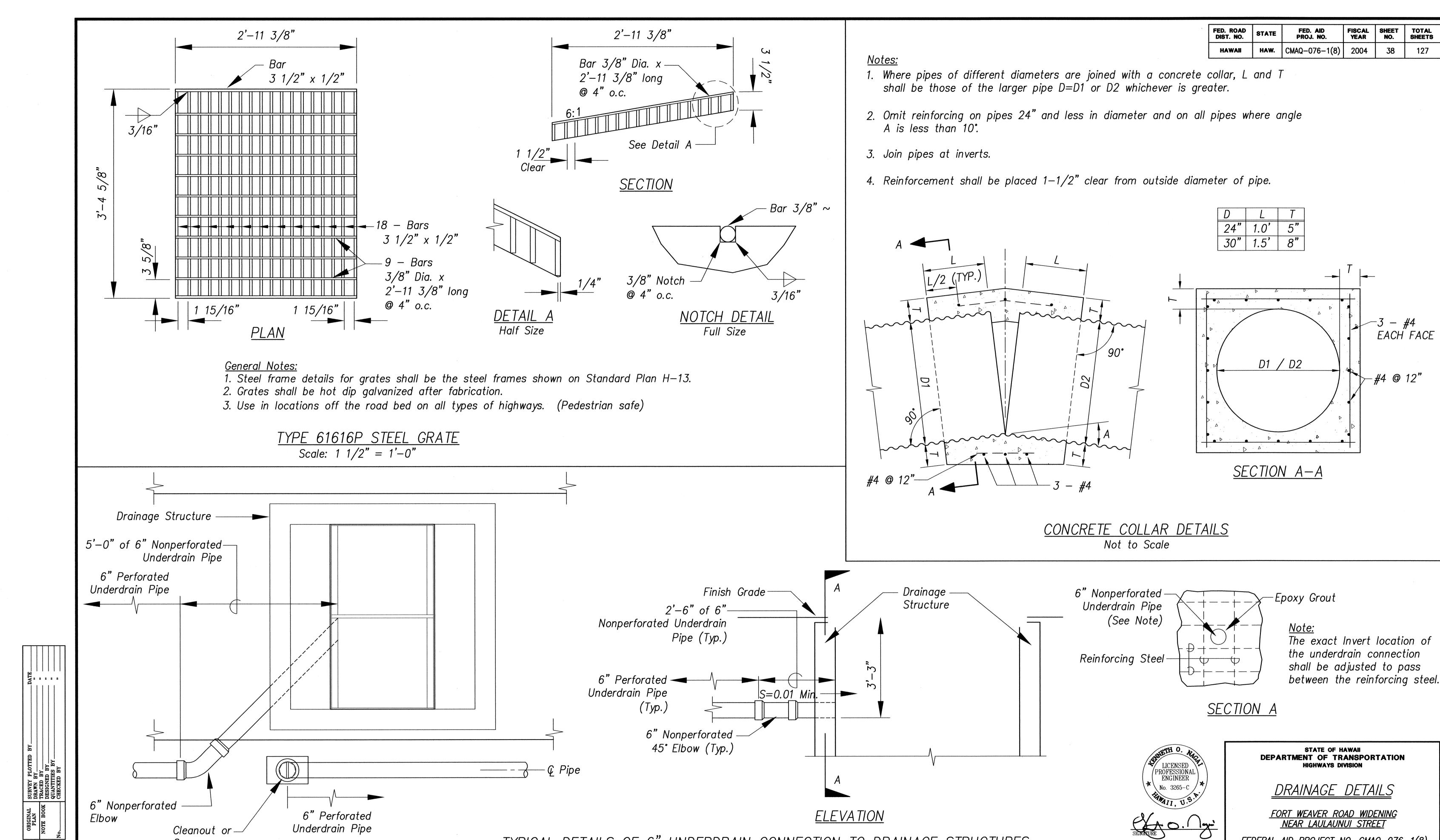
TYPICAL DETAILS OF 6" UNDERDRAIN CONNECTION TO DRAINAGE STRUCTURES
