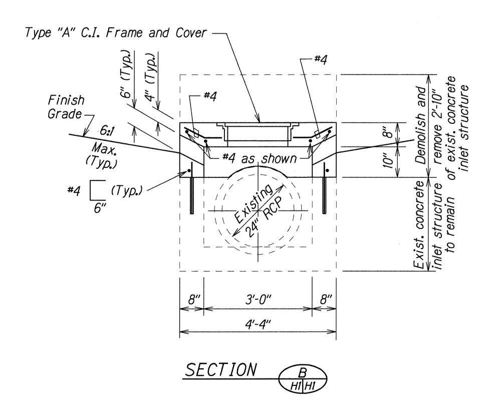
DETAILS OF MODIFIED TYPE "1" CATCH BASIN AT # STA. 224+40± RT.
