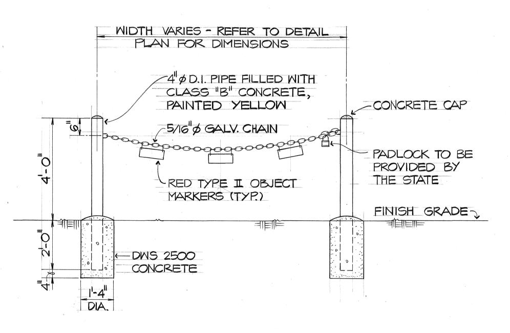
DRIVEWAY METAL POST & CHAIN DETAIL NO SCALE
