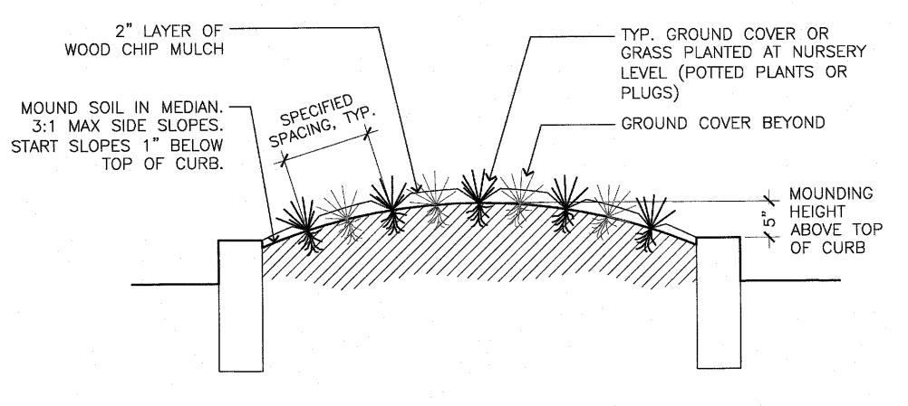
1. ON SLOPES, SET PLANT PERPENDICULAR TO SLOPE.
