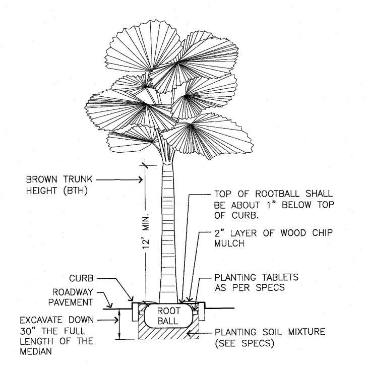
1. TRUNK TRUNK HEIGHT SHALL BE MEASURED FROM THE TOP OF THE ROOTBALL TO WHERE THE PALM FRONDS MEET THE BROWN TRUNK.
