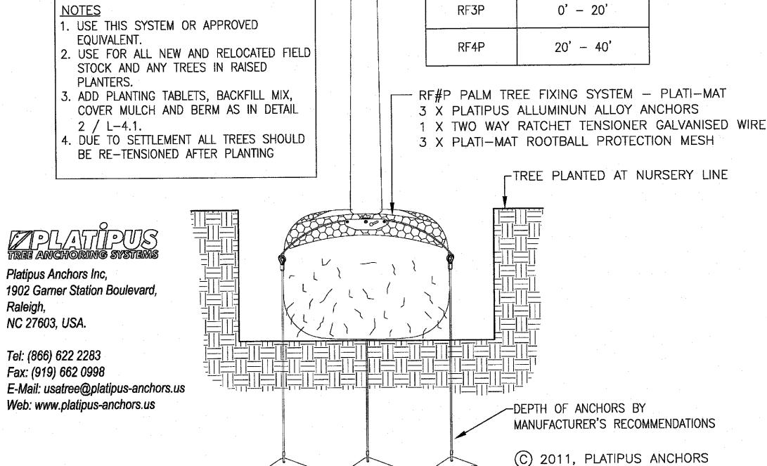
PALM UNDERGROUND STAKING DETAIL NOT TO SCALE
