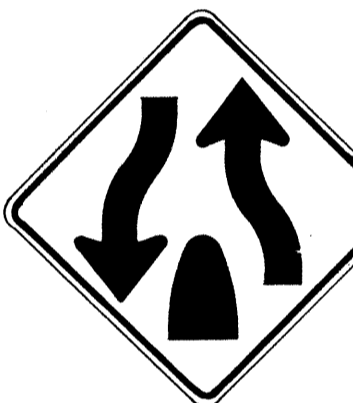
DIVIDED HIGHWAY ENDS
