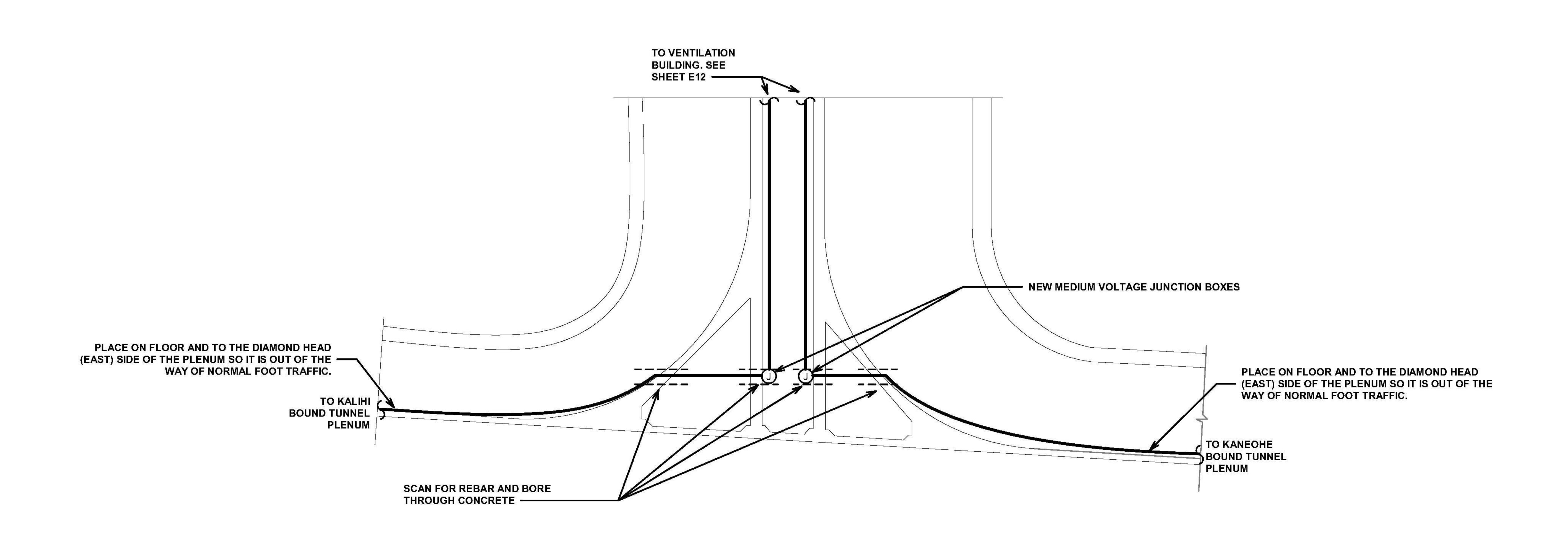
VENTILATION SHAFT/AIR PLENUM SECTION
