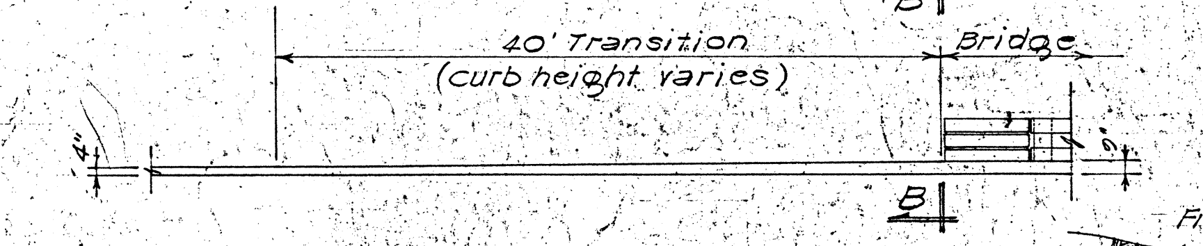
CURB ELEVATION 'A-A'
