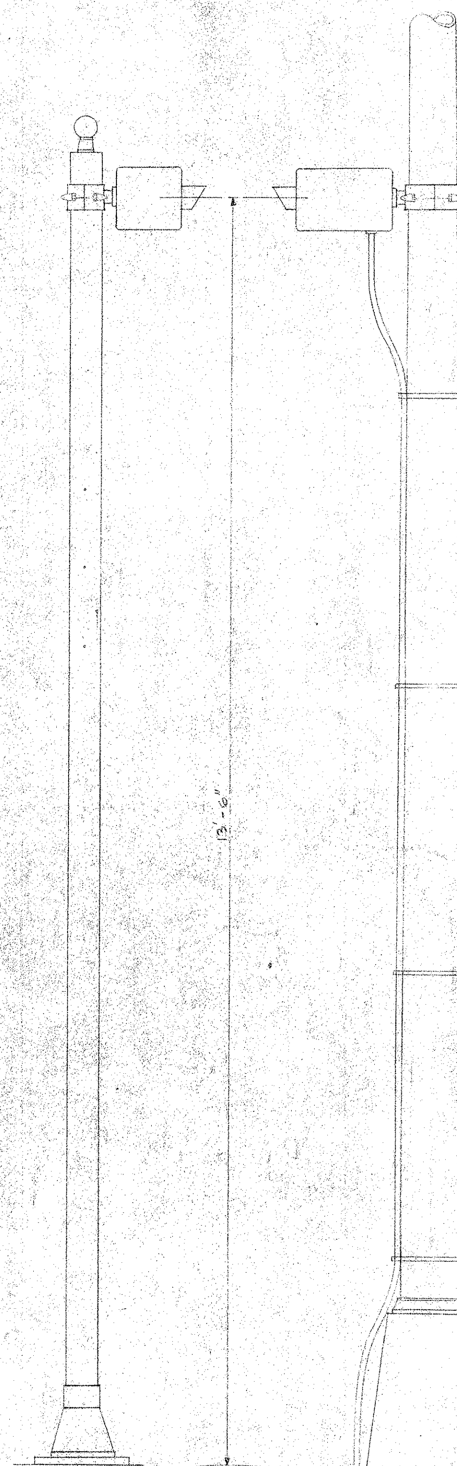
OVERHEIGHT ALARM PHOTOELECTRIC DEVICES ON 4\"/>
