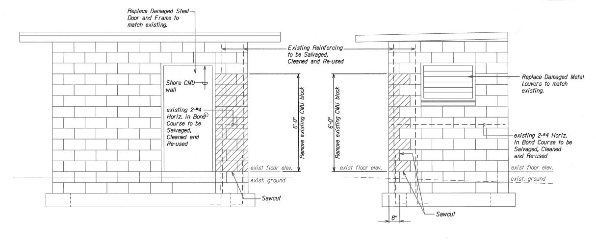
DEMOLITION ELEVATION A
