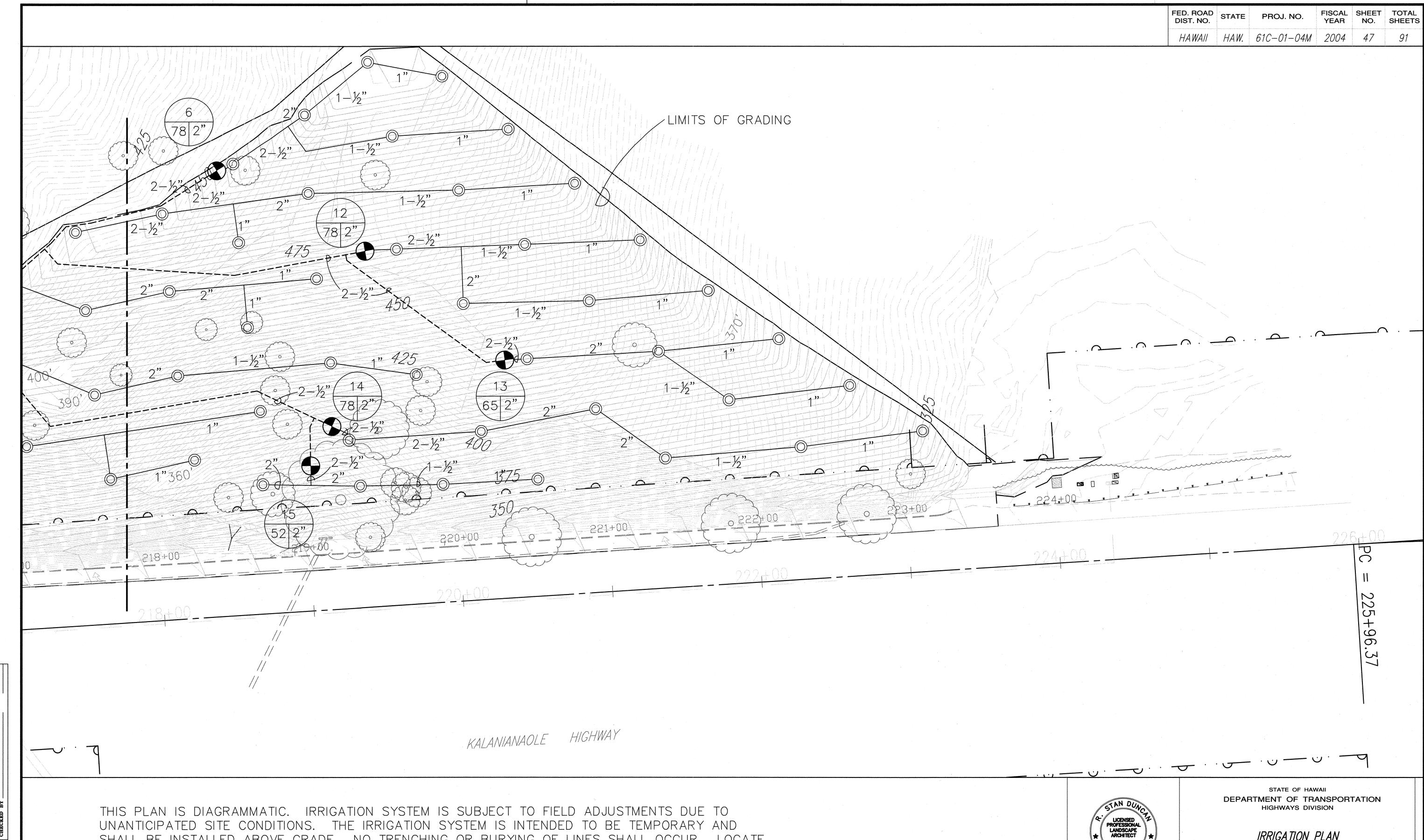
SHALL BE INSTALLED ABOVE GRADE. NO TRENCHING OR BURYING OF LINES SHALL OCCUR. LOCATE ALL MAINLINES, LATERALS, VALVES AND SPRINKLER HEADS WITHIN PLANTING AREAS, UNLESS OTHERWISE NOTED. AVOID ANY CONFLICT BETWEEN UTILITIES, STRUCTURES AND PLANTINGS. THE CONTRACTOR SHALL BE RESPONSIBLE FOR LOCATING AND PROTECTING ALL EXISTING UTILITIES.
