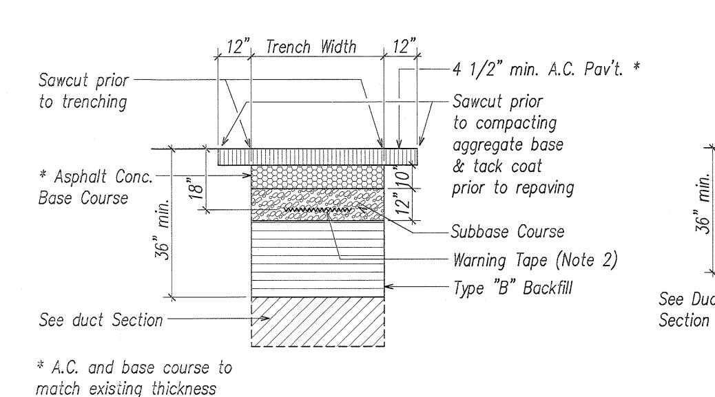
Mound 2" of top soil above finish grade, Trench Width Resod to match existing Aggregate subbase reg'd. if within 12" 10 ft. of pavement Warning Tape (Note 2) Type "B" Backfill See Duct
