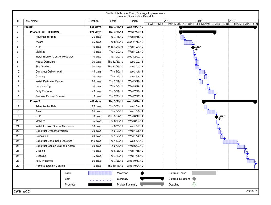
The project will be constructed in two (2) separate phases. The proposed improvements for Phase 1 and Phase 2 are shown in Figure 3 General Plan.
