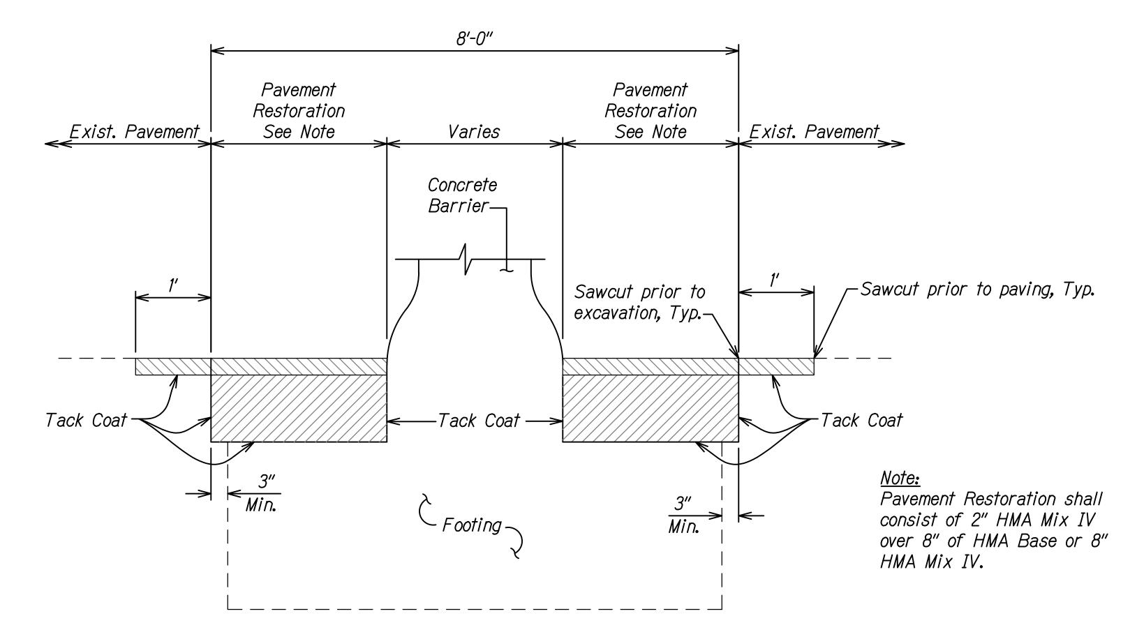
PAVEMENT RESTORATION DETAIL FOR SIGN H1ER-260 Scale: NTS
