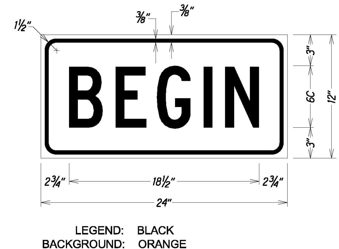
TYPICAL DETAIL FOR CONSTRUCTION SIGNS ON MULTILANE DIVIDED LOW SPEED HIGHWAY
