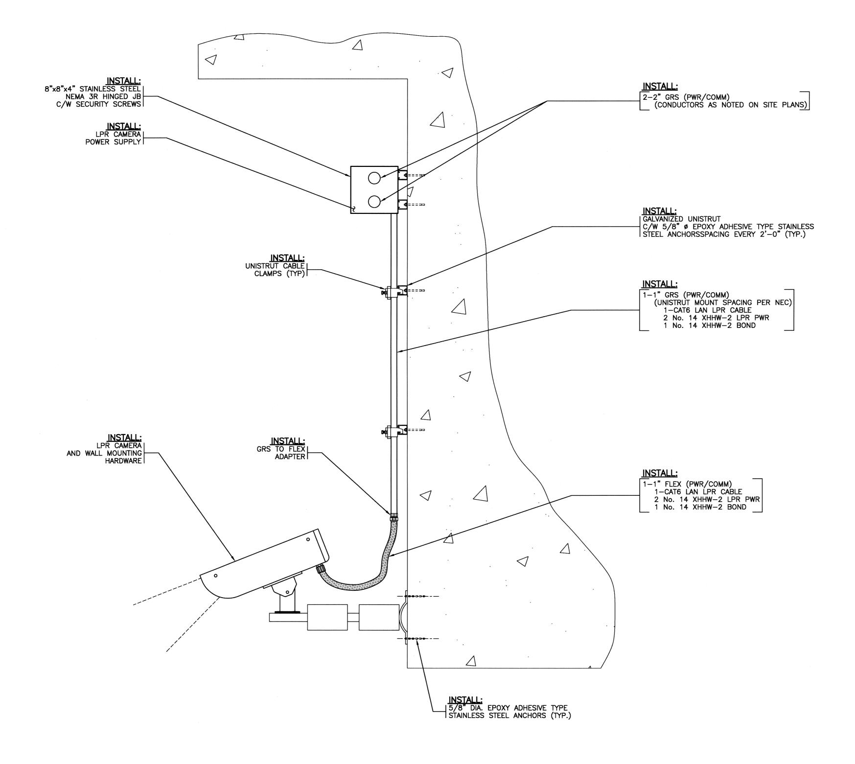
DETAIL 1 TYPICAL LPR CAMERA, CONDUIT AND JUNCTION BOX MOUNTING 2,5,8,12,15,16,20,24 29 N.T.S.
