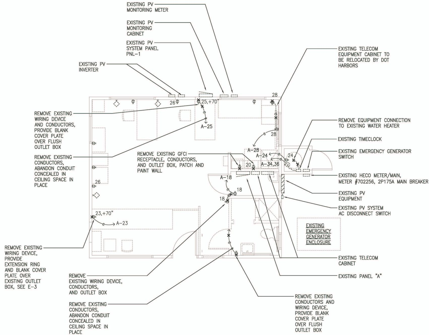
**1 ELECTRICAL DEMOLITION FLOOR PLAN**
