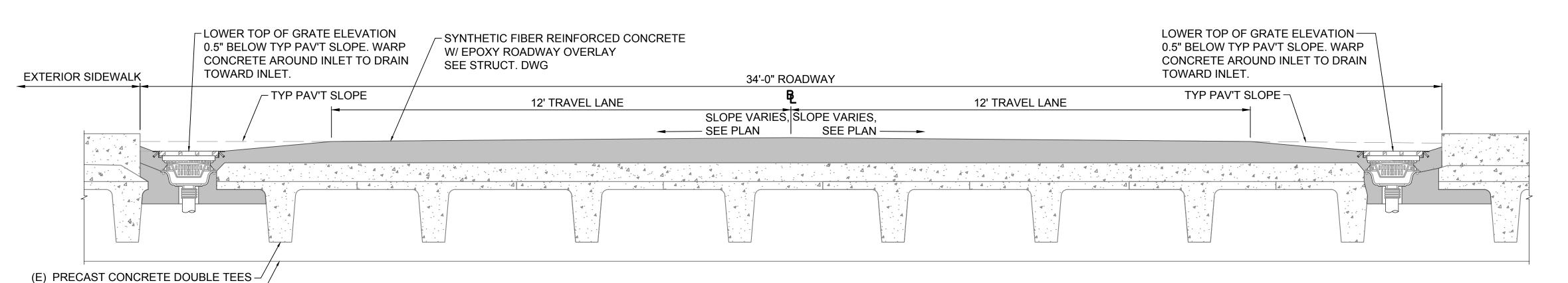
CROWNED ROAD SECTION AT DRAIN INLET STA. 6+82 TO STA. 14+57.50 (END)
