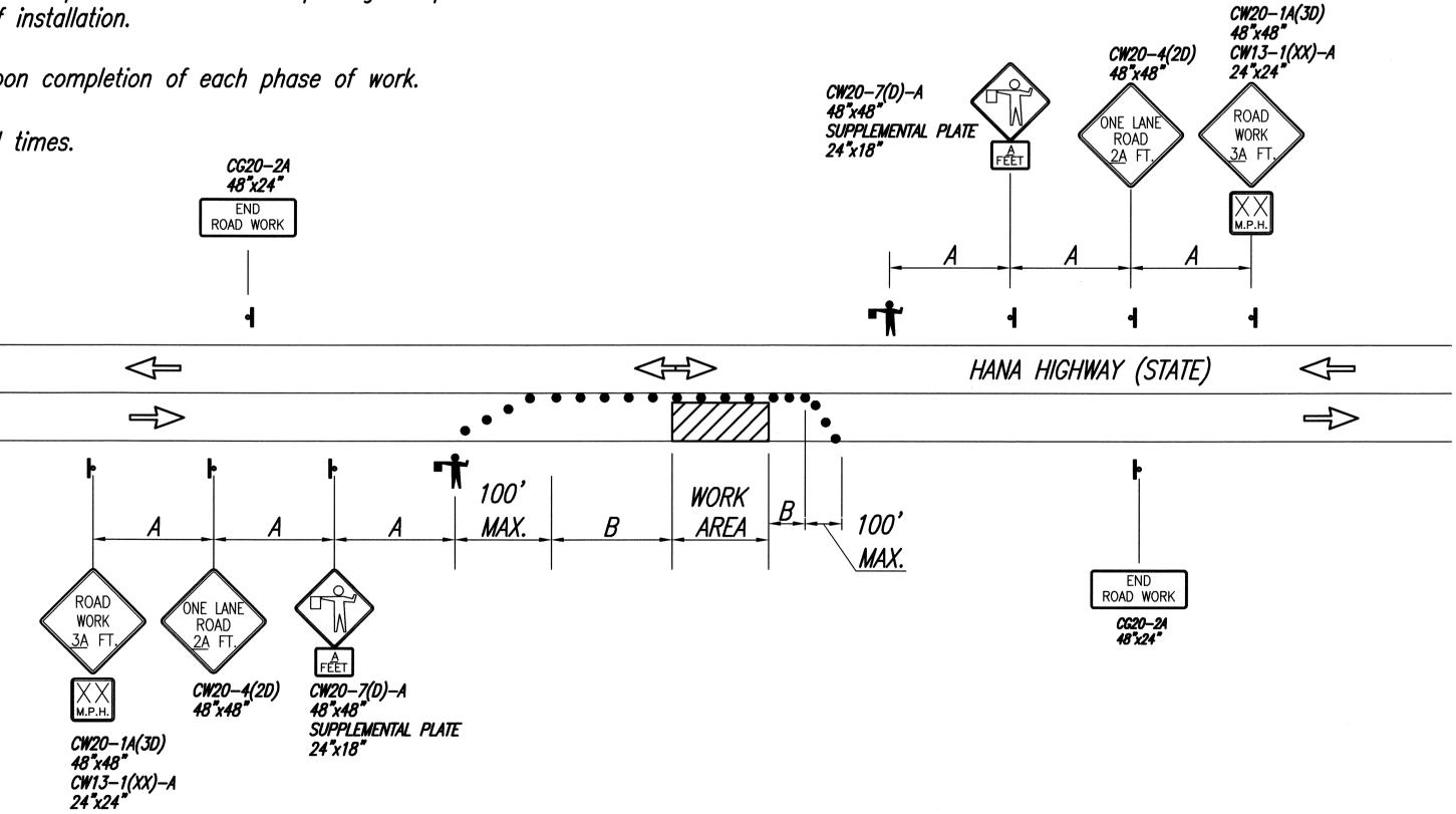
Traffic Control Plan <u>Two Lane Highway - One Lane Closed</u> Scale: NOT TO SCALE
