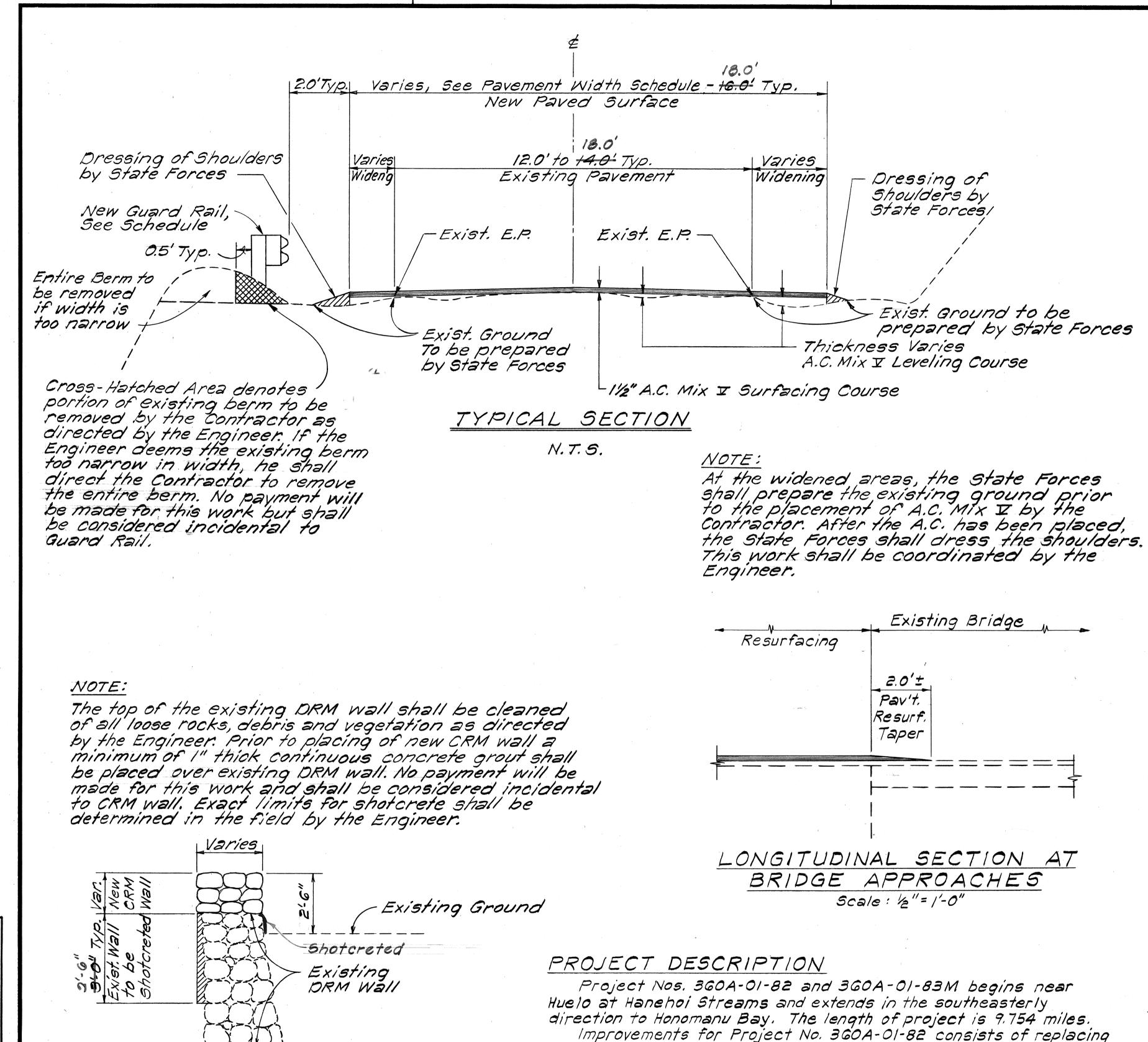
culverts, constructing CRM walls, shotcreting and installing
