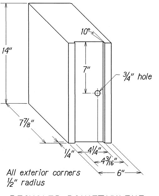
RECYCLED POLYETHYLENE OFFSET BLOCK (TYPE II)
