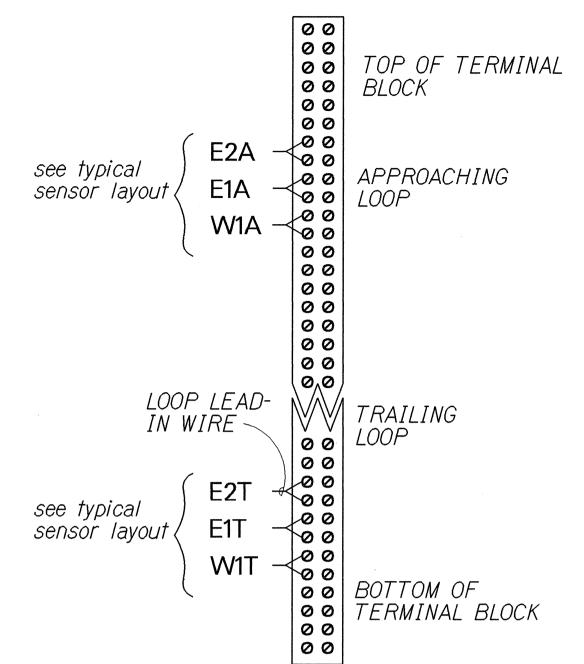
CONNECTING LAYOUT OF LOOP LEAD-IN WIRES TO TERMINAL BLOCK INSIDE JUNCTION BOX
