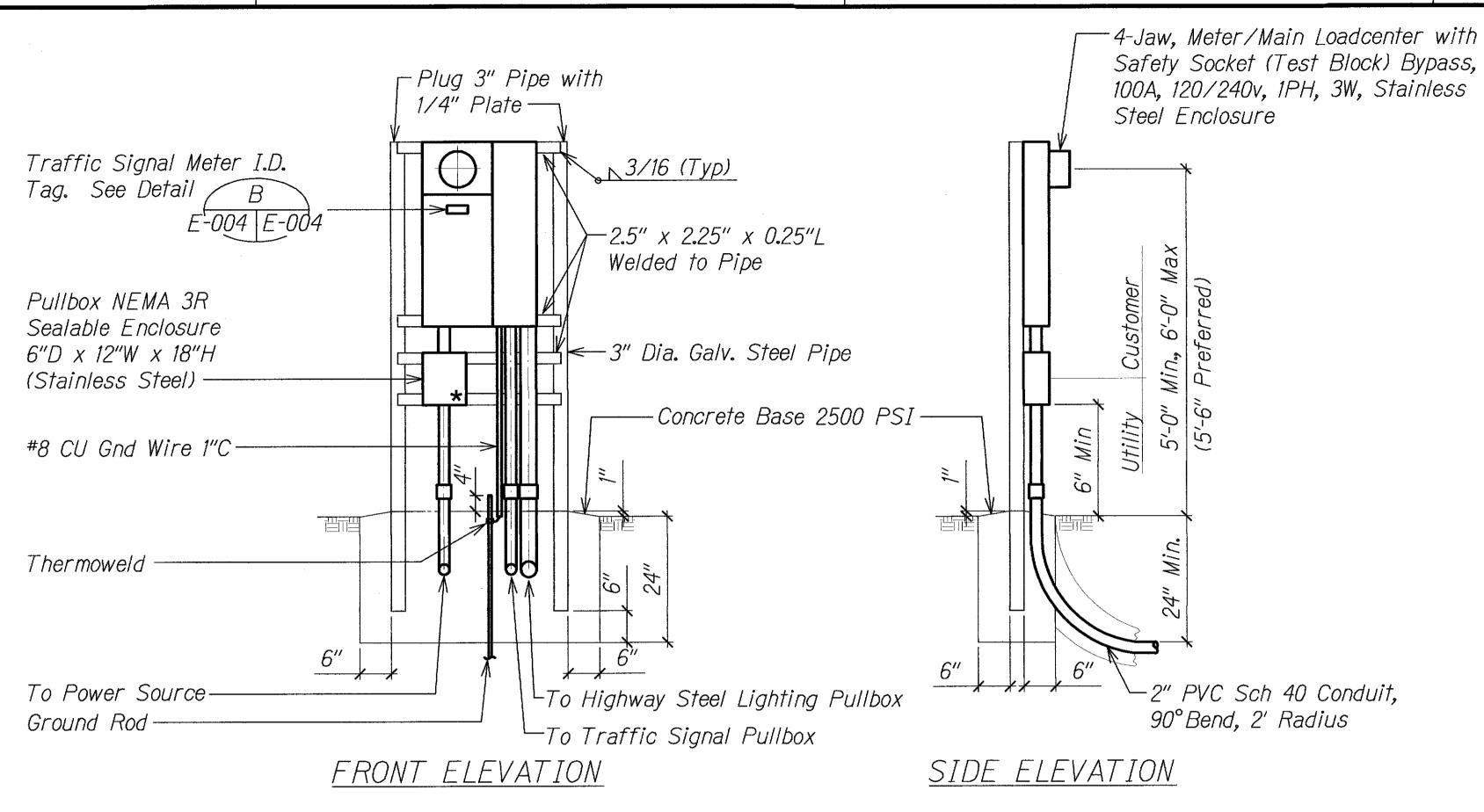
A METER PEDESTAL FOR UNDERGROUND SERVICE E-004 E-004 NTS
