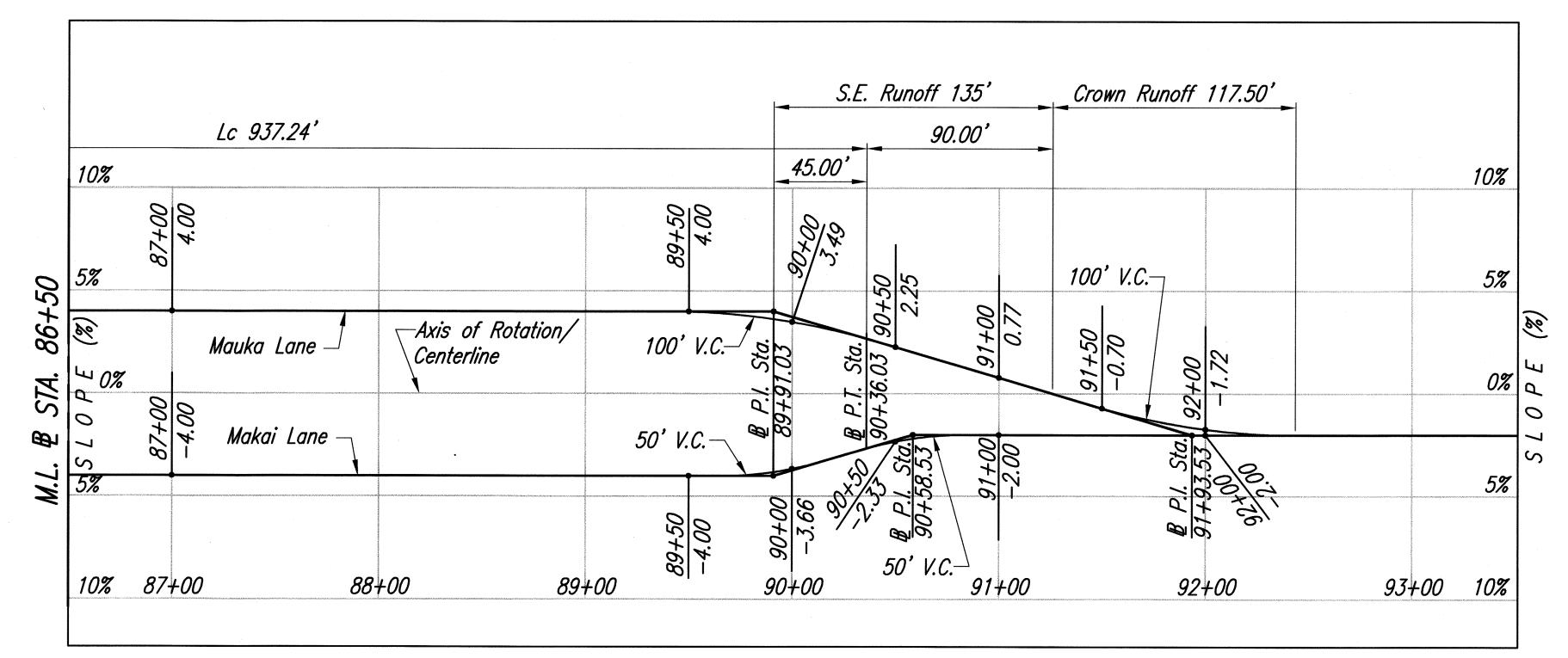
SUPERELEVATION DIAGRAM Scales: HORIZ. 1"=40' VERT. 1"=4%
