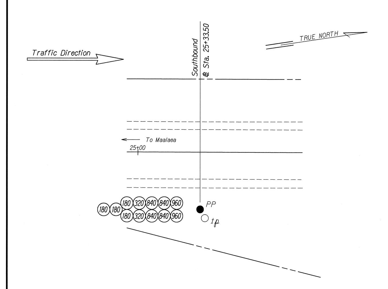
TEMPORARY CRASH ATTENUATOR FOR MECO POWER POLES Not to Scale
