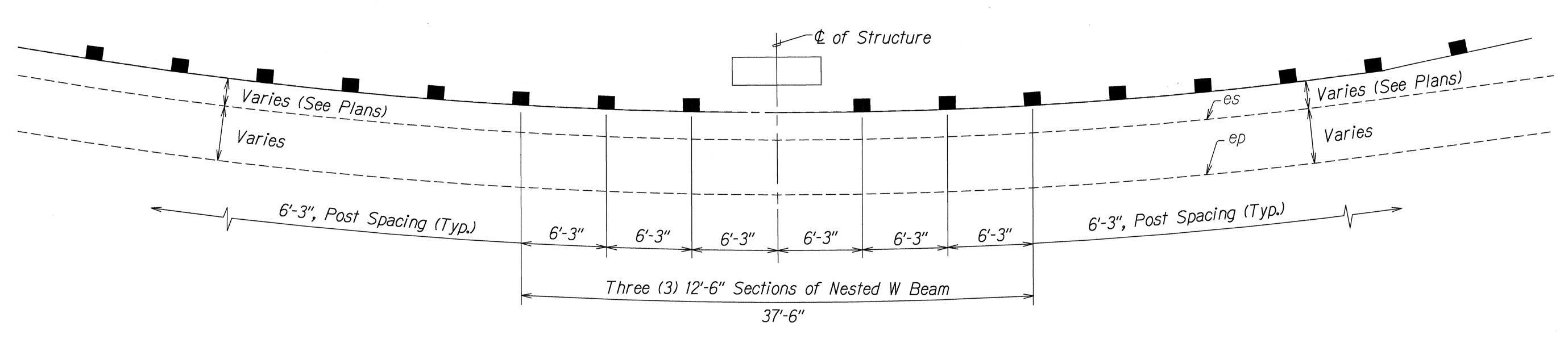
Note: All work associated with the Nested W Beam shall be incidental to Guardrail, Type 3 - Double Nested with Steel Post. This work shall be approved and as directed by the Engineer.
