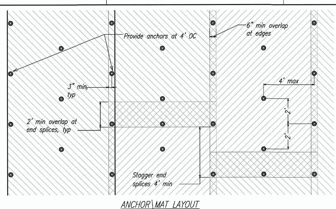
FED. ROAD STATE HAW. MAUI Erosion mat -Anchor Plate - Conical Wedge Grip Stainless Steel Tendon --Slight depression Mechanical earth anchor (Platipus S4 Geo or equal) Install per manufacturers' instructions Notes: Secure all erosion mat edges with mechanical earth anchors at 4' on center.
