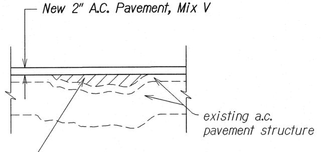
Fill Depressions in existing A.C. Pavement with leveling course of A.C. Pavement Mix No. V. Locations and size, if any, determined on the field by Engineer during construction
