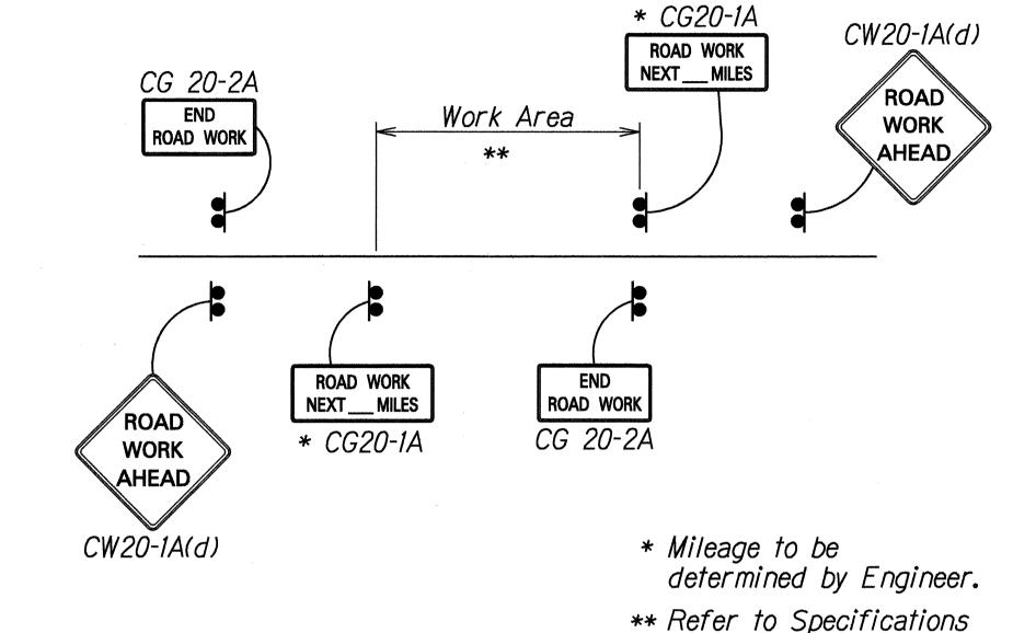
plan. PERMANENT CONSTRUCTION SIGN LAYOUT DETAIL
