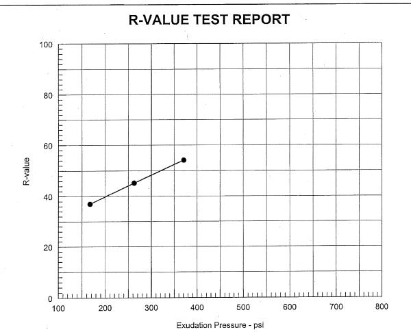
Resistance R-Value and Expansion Pressure - ASTM D 2844
